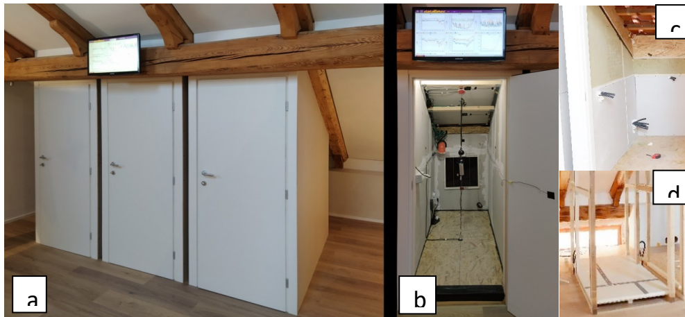
Fig. 1 a) The three test rooms; b) Internal view and sensors position; c) Construction of walls d) Construction of floors
